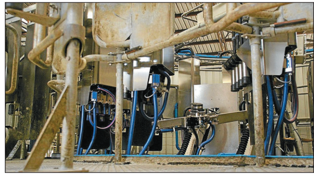
The robotic arm on the prototype robotic rotary dairy at FutureDairy's Camden, NSW, research farm.
